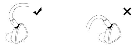
When wearing the earphones, gently rotate and press the units according to the direction shown in the picture. After properly wearing, put the earphone cable over your ear and adjust the earphones until you feel comfortable.
