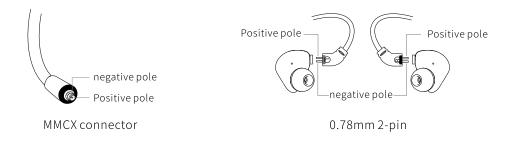
This product adopts an over-the-ear wearing design. When installing the earphone cable, please ensure the earphone unit and cable form a shape that can wrap around the ear as shown in the figure below.
