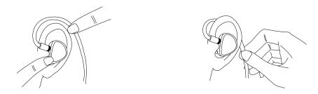
When removing the earphone cable, hold the cable connector and the earphone unit tight with your fingers. Keep them in the same line and then pull them apart. Or use the MMCX assist tool to detach it (Please refer to the instruction of the MMCX assist tool to see how to use it). Note that do not rotate the 0.78mm 2-pin cable.
