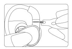
① Align the semi-circular indentation of the MMCX assist tool to the gap between the connector's male and female components.
