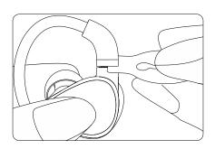
② Ensure the tool is parallel to the gap and position it towards the gap between the connector's male and female components until it is in place.
