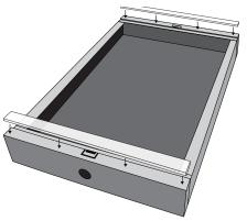
For plasterboard thinner than 12.5mm (1/2") Shim adhered to Backbox
