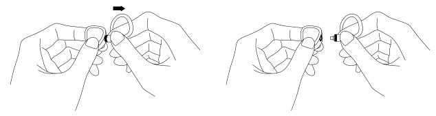
Please do not install or remove the cable at a tilted angle, and do not pull the earphone cable directly, so to avoid it being broken.
