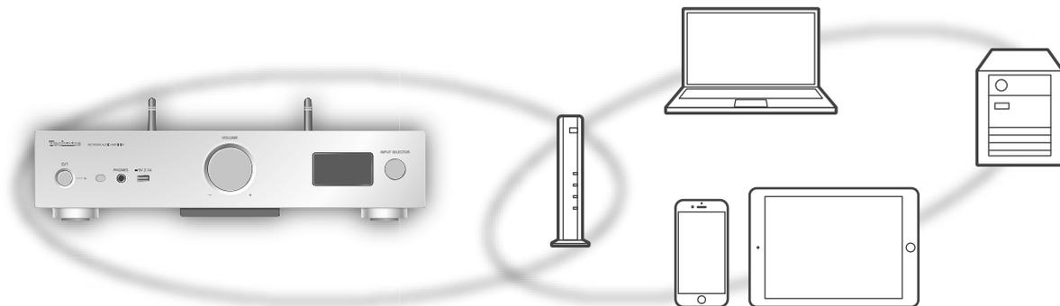
This system can be connected to a router using a LAN cable or built-in Wi-Fi®. For a stable connection to the network, a wired LAN connection is recommended.
