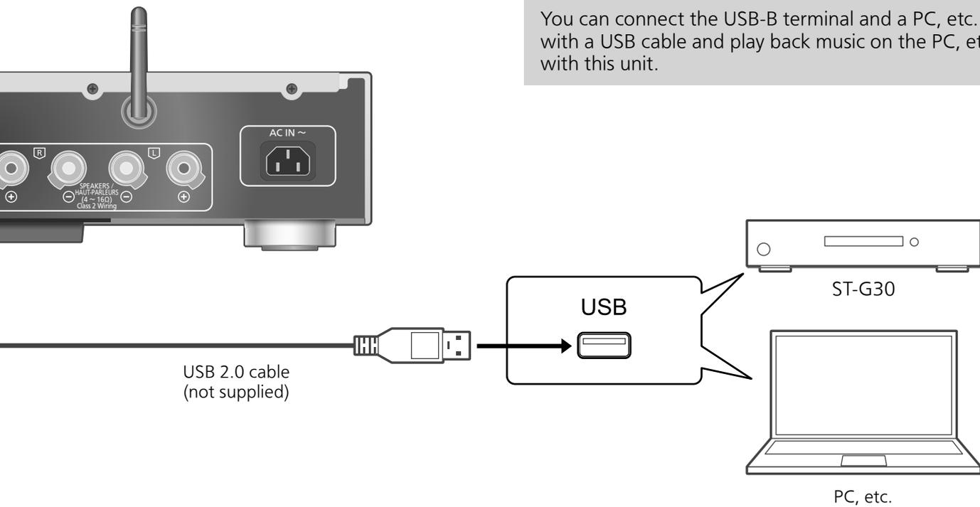
You can connect the USB-B terminal and a PC, etc. with a USB cable and play back music on the PC, etc. with this unit.
