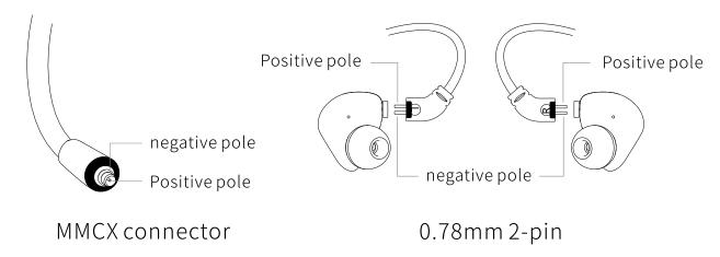
This product adopts over-the-ear wearing design. When installing the earphone cable, please make the earphone unit and cable form a shape that can wrap around the ear, as shown in the figure below.
