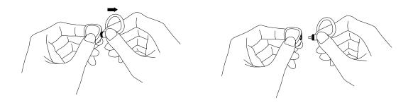
Do not install or remove the cable at a tilted angle. Do not pull the earphone cable directly, to avoid it being broken.
