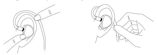
When removing the earphone cable, hold the cable connector and the earphone unit tight with your fingers. Keep them in the same line and then pull them apart. Note that do not rotate the 0.78mm 2-pin cable.
