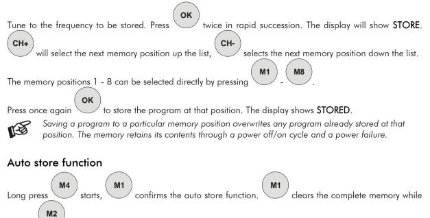
storing. keeps stations with good signal strength in the memory and overwrites stations with insufficient signal level while storing.
