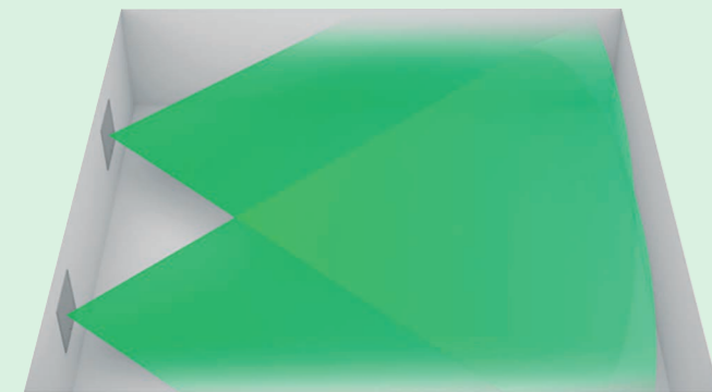
DALI Wide Dispersion design principle
